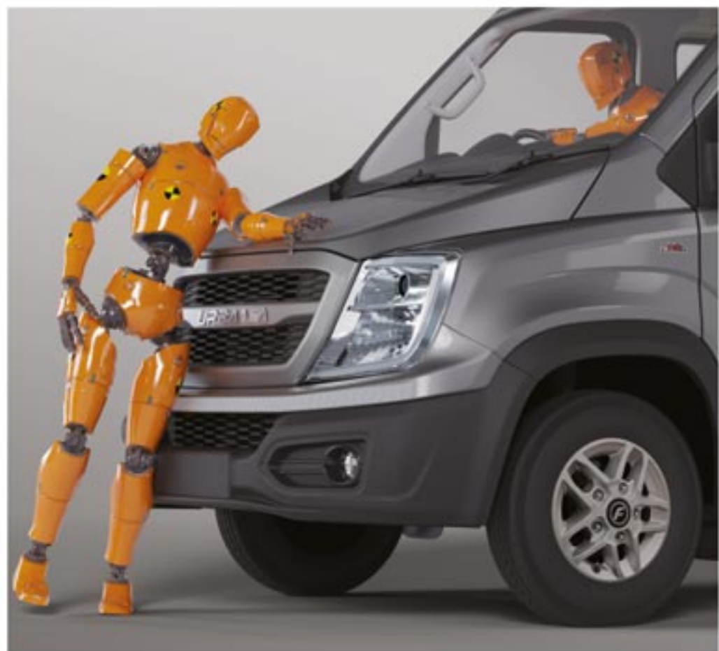
Front Bumper Designed to Minimise Pedestrian Injury
